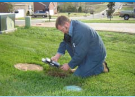
Michael Clay from the West Wilson Utility District profiles a customer's meter using the Badger ® -Radix ® handheld.
