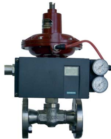
Siemens Sipart PS2 mounted on 1/2" Type 754
