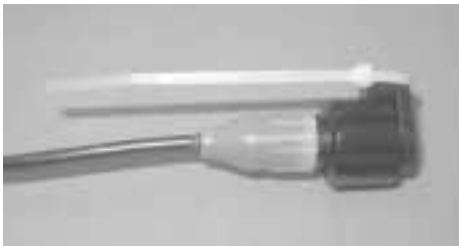
Cable Tie on Register or Reed Switch Connector
