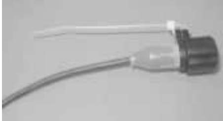
Cable Tie on ERT Connector
