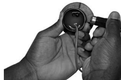
Figure 4 - Activation of Badger® GALAXY® Pit Transmitter
