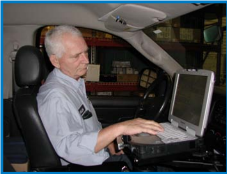
Keith Solomon using the ORION ® laptop and software to read the city's meters as he drives by.
