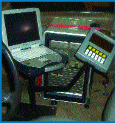
Pictured above is the ORION ® premium reading system along with the TRACE ® Mini Mobile Interrogator used in the City of Red Bluff's water utility vehicle.
