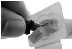
Gel Connectors Going into Field Splice Tube Gel Connectors Inserted into Field Splice Tube
